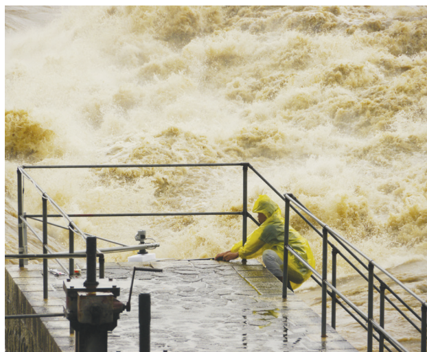
Technician testing a radar water level sensor in early warning system supported by GIZ in Phu Yen Province
