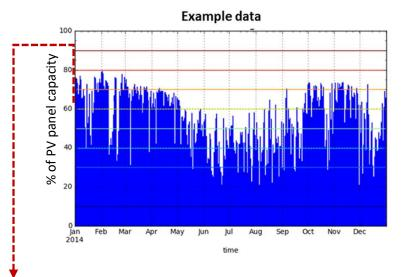
Capping the inverter somewhere here would reduce peak feed-in while losing only a small amount of yearly energy.
