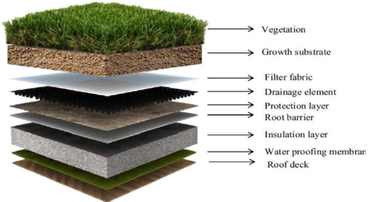
Figure 4.9: Green roof design
